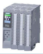
SIMATIC S7-1500 compact CPU, CPU 1512C-1 PN, central processing unit with work memory: 400 KB for program and 2 MB for data, 32 digital inputs, 32 digital outputs, 5 analog inputs, 2 analog outputs, 6 high-speed counters, 4 fast outputs for PTO/PWM/frequency output, 1st interface: PROFINET IRT with 2-port switch, 6 ns bit performance, including front connector push-in, SIMATIC Memory Card required
