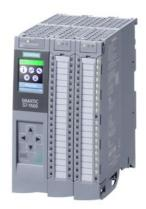
SIMATIC S7-1500 compact CPU CPU 1511C-1 PN, central processing unit with 300 KB work memory for program and 1.5 MB for data, 16 digital inputs, 16 digital outputs, 5 analog inputs, 2 analog outputs, 6 high-speed counters, 4 high-speed outputs for PTO/PWM/frequency output 1st interface: PROFINET IRT with 2-port switch, 6 ns bit performance, including front connector push-in, SIMATIC Memory Card required
