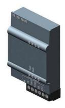
SIPLUS S7-1200 CB 1241, based on 6ES7241-1CH30-1XB0 with conformal coating, -40...+60 °C, start up -25 °C, RS-485, terminal block, supports Freeport
