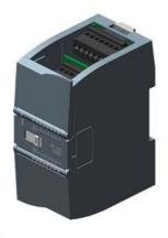
SIPLUS S7-1200 SM 1223 8DI/8DQ/relay based on 6ES7223-1PH32-0XB0 with conformal coating, -40...+70 °C, start up -25 °C, digital input/output 8 DI/8 DQ, 8 DI 24 V DC, sink/source, 8 DQ, relay 2 A
